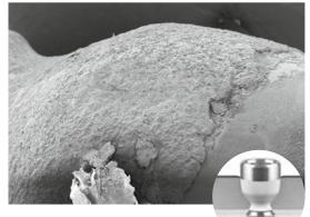
SEM images of retrieved abutments show that only the DermaLock surface (unlike all-titanium abutments) is capable of binding with viable soft tissue.<sup>7</sup>
