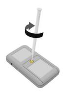
Lock the battery cover in place by turning the screw clockwise with a small Phillips head screwdriver until tight.
