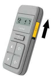
When the switch is in the up position, the remote control will "go to sleep" when not in use. Press any button to "wake" it again.
