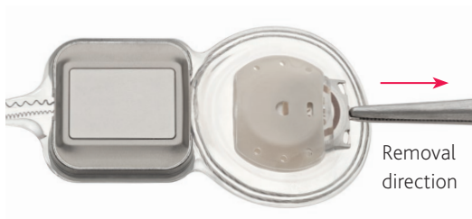
Figure 29: CI632 implant, magnet cassette removal using metal tab
