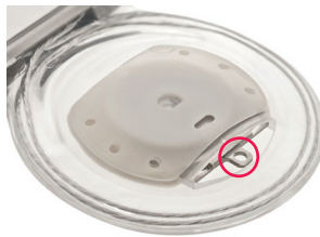
Figure 19: Metal tab on magnet cassette
