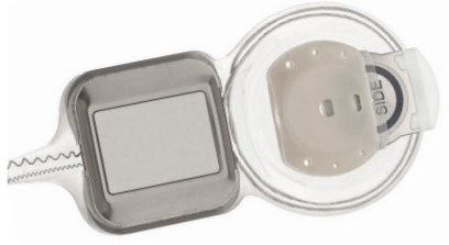
Figure 1: CI612 cochlear implant with magnet cassette partially removed from pocket
