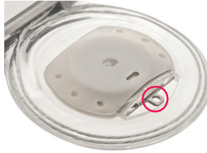
Figure 25: Metal tab on cassette
