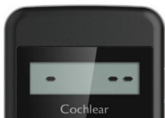
If your remote control is not paired to any processor, it displays dashes (shown left) and “blinks” when you press buttons.
