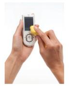
Figure 64: Wiping the remote assistant with a soft dry cloth
