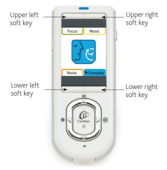
Figure 17: Soft keys for selecting a program from Home screen
