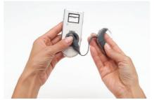
Figure 12: Placing the coil on the coil sensor guides
