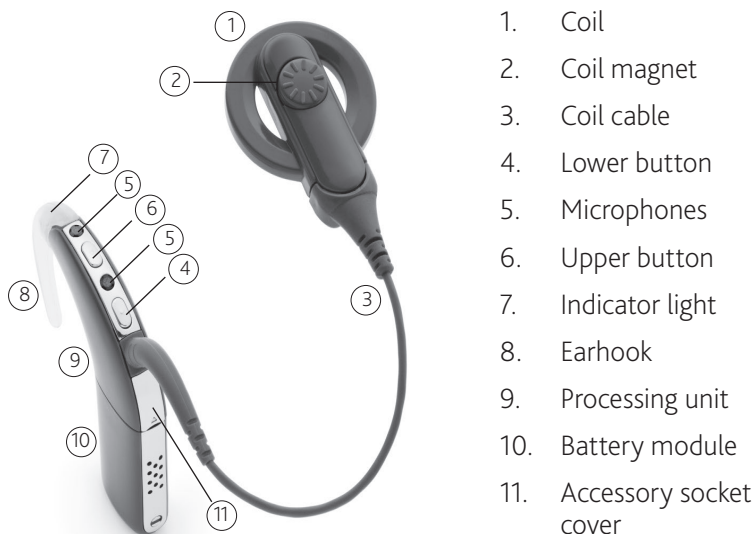
Figure 1: CP810 Sound Processor parts
