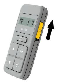
Slide the switch up to turn on.
