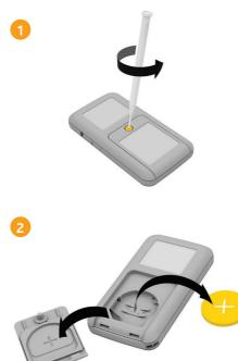
Unlock the battery cover by turning the screw anticlockwise with a small Phillips head (cross-head) screwdriver.
