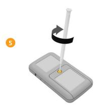
Lock the battery cover in place by turning the screw clockwise with a small Phillips head screwdriver until tight.
