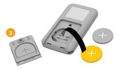
Insert the new battery. Make sure the plus sign "+" is facing up. Take care not to damage the battery contacts.
