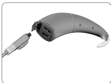
Plugging an accessory into the accessory socket
