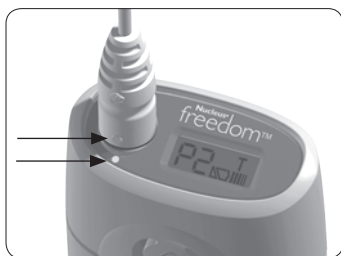
Dots lined up on connector and controller
