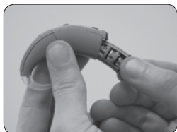
Replace the battery rack.
