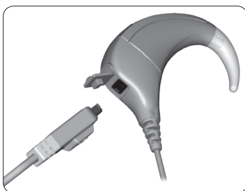
Plugging an accessory into the accessory socket
