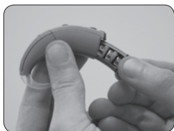
Remove the battery rack.
