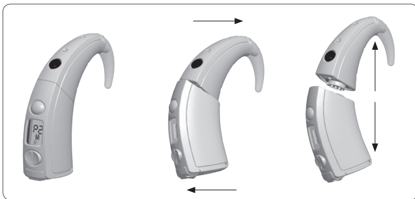
Removing the Processing Unit from the BTE Controller
