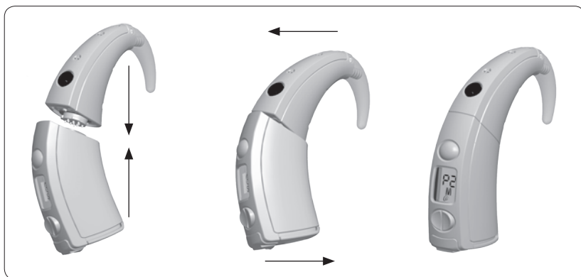
Attaching the Processing Unit to the BTE Controller
