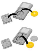
Slide off the battery cover and remove the battery.
