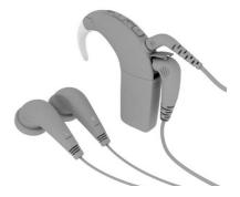
Carers can use a monitor earphone to check that the processor and plug-in audio accessories are receiving sound.
