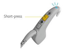
Short-press the upper button to switch between microphones and the plug-in audio accessory.
