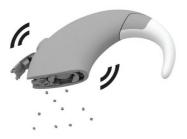
If sand or dirt ever enter the processor, shake the components carefully to remove it and change the microphone protectors.
