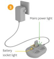
Connect the battery charger to the power adaptor and plug into mains power.
