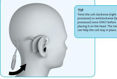
processor) or anticlockwise (left processor) once ONLY before placing it on the head. The twist can help the coil stay in place.
