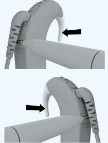
To increase tamper resistance, push the lock to the far left with your battery cover locking tool to lock the battery module.
