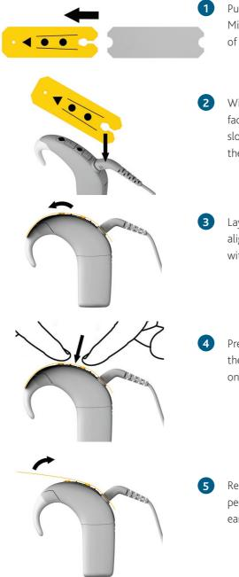
Pull the Cochlear<sup>™</sup> Nucleus<sup>®</sup> Microphone Protector Applicator out of its sleeve.
