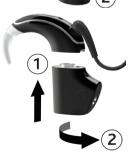
Insert the monitor earphone adaptor, then twist to connect.
