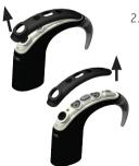
2. Lift the microphone cover from the bottom edge, then lift it up to remove.
