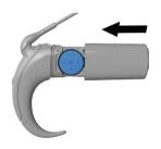
Replace the battery cover by sliding it up towards the processing unit.
