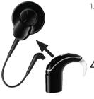
Hold the coil cable grip and firmly pull it straight out of the processor.
