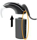
2. Twist the battery module as shown to attach the parts.
