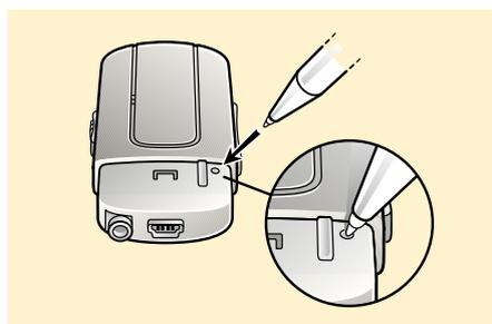
**D** The LED will flash yellow every 2 seconds and the Mini Microphone will now be in pairing mode for 20 seconds.
