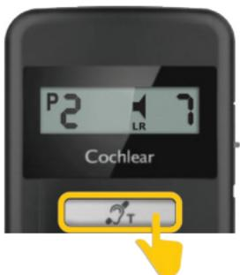
2. To stop streaming audio, short-press the telecoil button.
