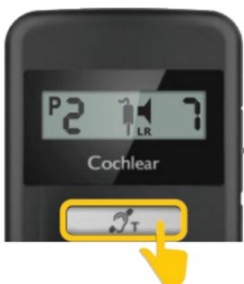
1. To start streaming audio, press and hold the telecoil button for 2 seconds, then release.
