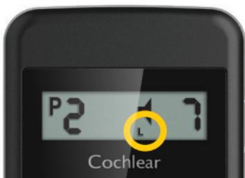
5. The remote control then shows successful pairing of either left (L) or right (R) processor.
