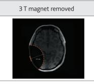
The image artefact extends 5.7 cm (2.2 in.) from the centre of the CI512 cochlear implant when using a gradient echo pulse sequence scan.
