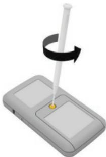
1. Unscrew cover with a Phillips head (cross-head) screwdriver.
