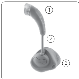
Acoustic Component: with earhook (1), cable (2) and earpiece (3)
