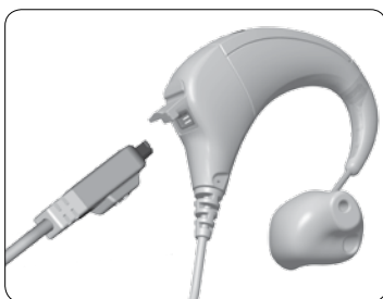
Plugging an accessory into the accessory socket
