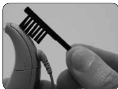
Cleaning the microphone protector
