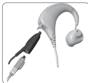
Testing an accessory with the monitor earphones
