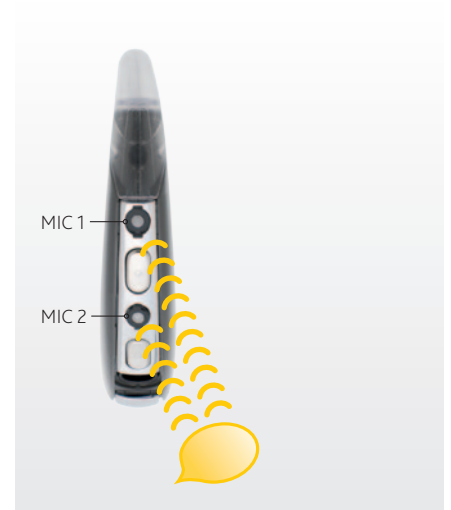
Sounds from behind arrive at MIC 2 first then at MIC 1 second.
